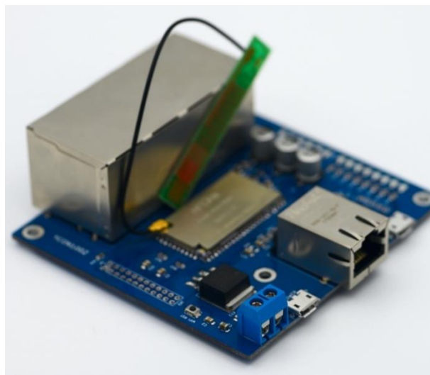
Figure 17: Xetal Yugen Hub used to aggregate data from several sensors and upload it to the Yugen Fusion Server.
