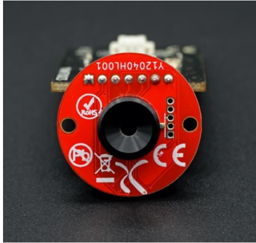
Figure 16: Latest Xetal Yugen prototype (40x120 FoV) including a wireless module connected to its back.
